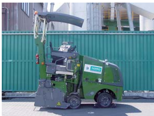
Photo 3-2: Rumble strip installation machine (high-performance model)
