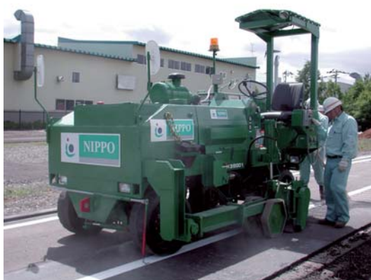
Photo 3-3: Rumble strip installation machine (for road shoulders)
