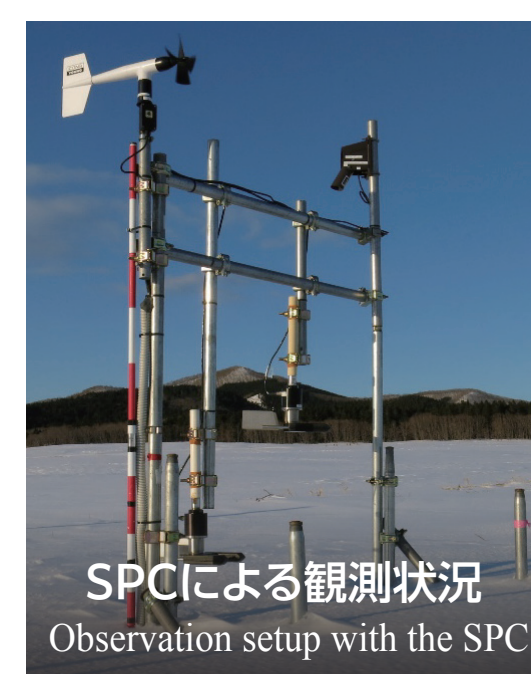
Fig. 6 Snow transport observation at locations with different fetches (Teshikaga Town, Hokkaido Prefecture)
