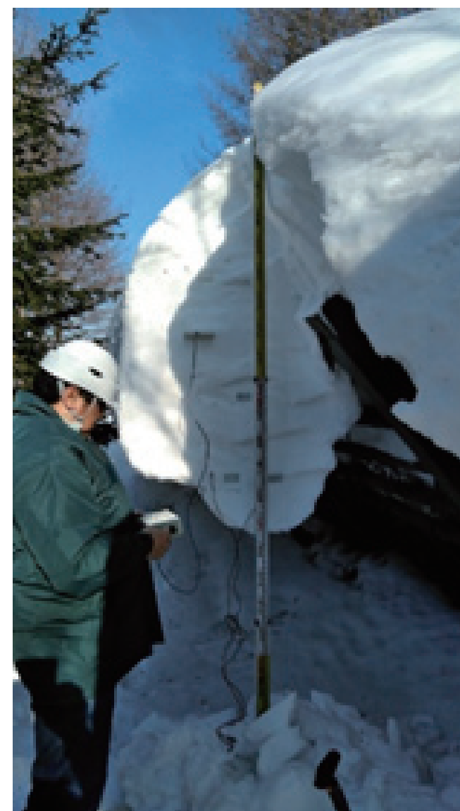
▲図1: 巻きだれ断面の観測状況 (2019.3.18) Fig. 1 A researcher observes the cross-section of a snow eave. (2019-3-18)
