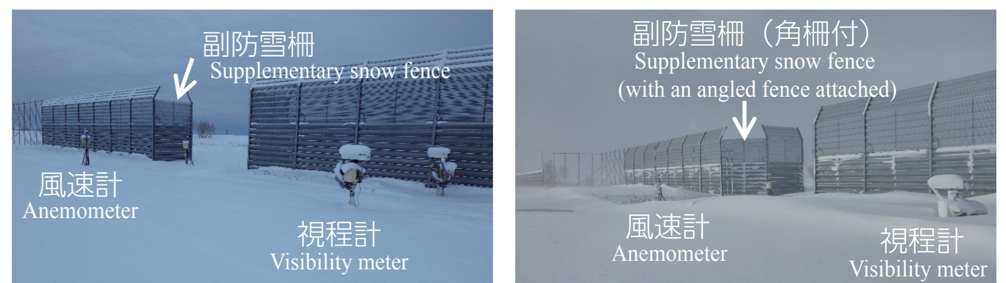
▲L字型副防雪柵の現地観測 Onsite observations of an L-shaped supplementary snow fence
