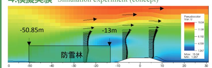
▲模擬実験を活用した防雪林の評価(イメージ) Evaluation of snowbreak woods that are designed based on the results of the simulation experiment (concept)
