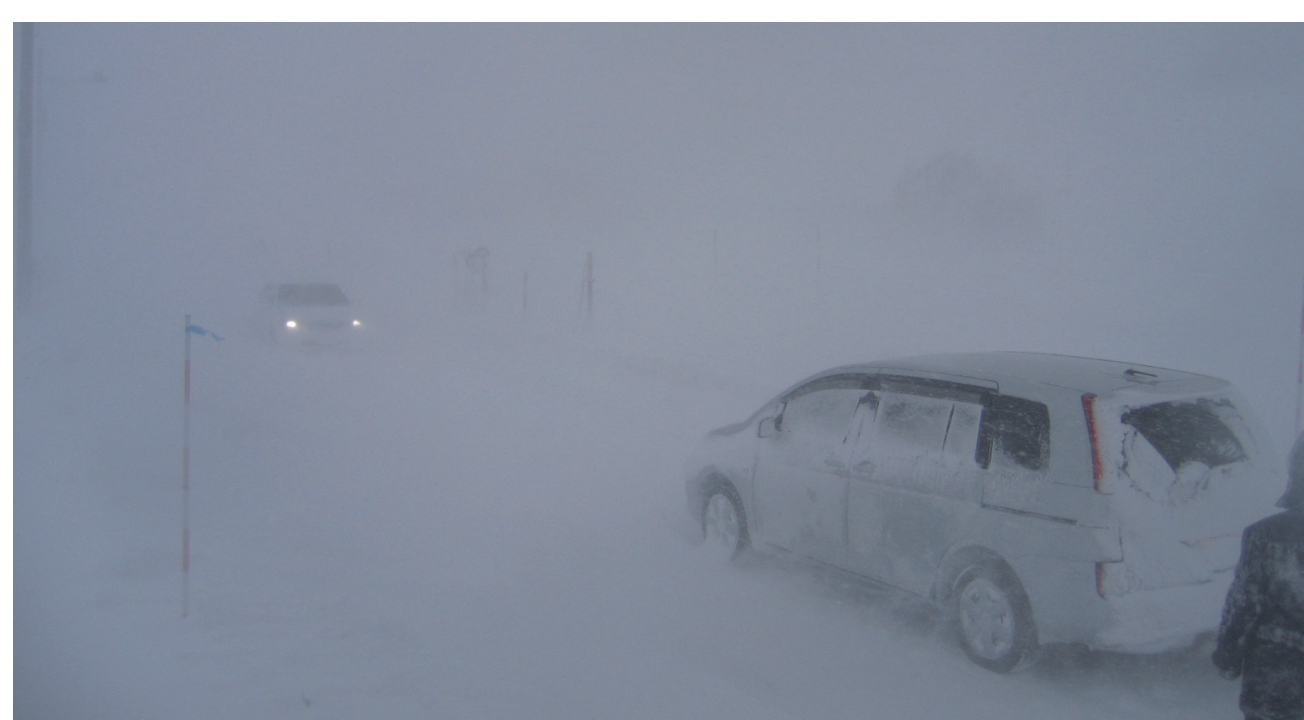
視線誘導施設や車両の視認性調査 Test on visibility of several types of delineators and cars in blowing snow
