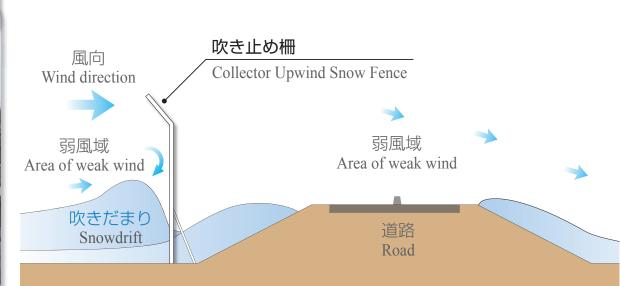
There are three major types of snow fences: collector snow fences, blower snow fences, and collector upwind snow fences. In addition to these three types, "solid barriers" for preventing snow from blowing onto the road from valleys are also used.
