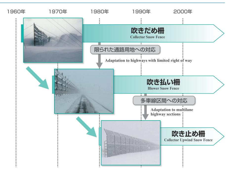
▲吹きだまりから視程障害への目的の変化に応じた防雪柵 Snow fences have been changed in response to the shift in objectives from snowdrift control to poor visibility mitigation.
