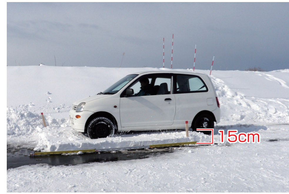
▲吹きだまり深さ 15cm：発進可能 15cm-deep snowdrift: Starting from a standstill is possible.
