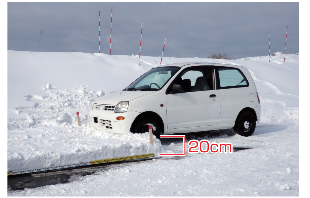
▲吹きだまり深さ 20cm：発進不能 20cm-deep snowdrift: Starting from a standstill is impossible.
