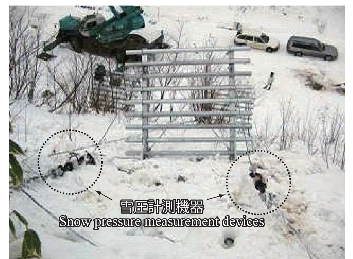
▲雪圧の測定方法 Measurement of snow pressure on the snow bridge
