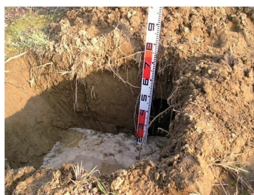
▲生育不良木周辺地盤の滞水状況 Excessive moisture in the ground around poorly growing trees
