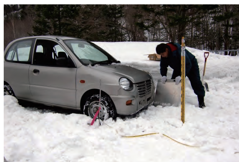
▲自動車の走行限界に関する実験(写真：吹きだまり高さ15cmの例) Experiment on the limit of a vehicle's ability to travel through snowdrifts (Photos: experiment at 15-cm-deep snowdrifts)
