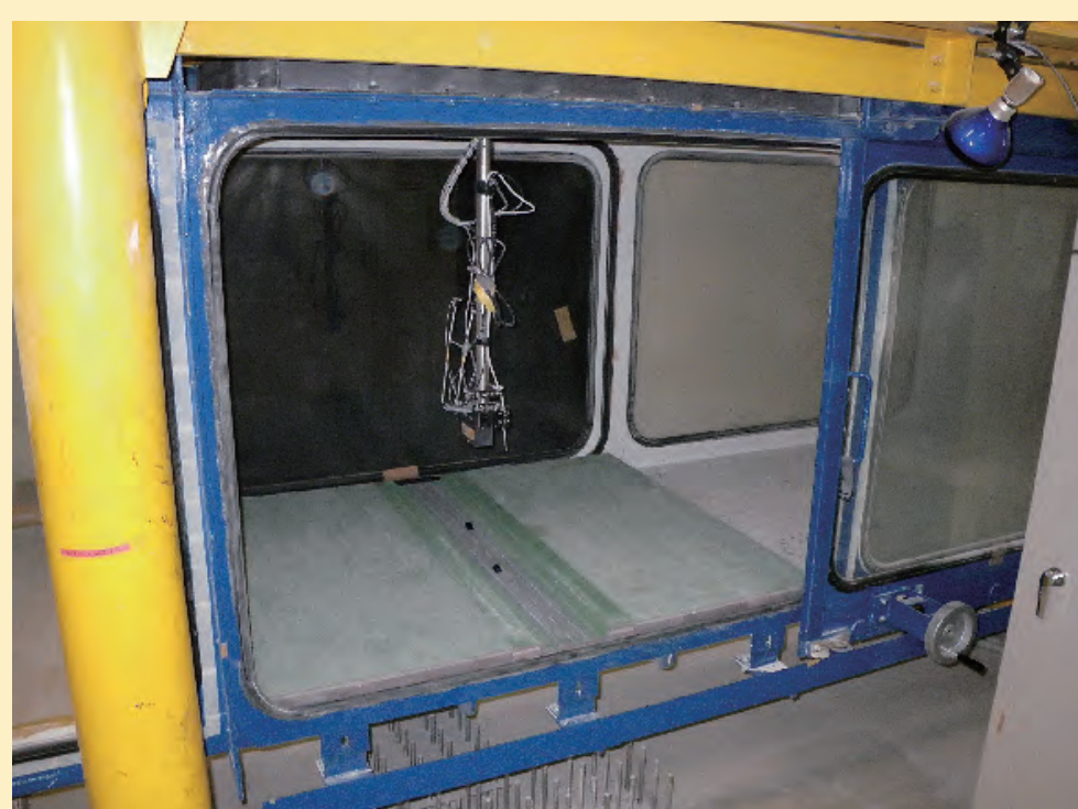
▲風洞測定洞部分(寸法：L=6.0m×W=1.2m×H=1.2m) Test section of the wind tunnel (Dimensions: L=6.0 m, W=1.2 m, H=1.2 m)
