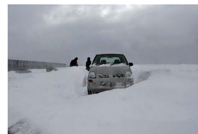
▲吹きだまりの発生状況の観測(左：切り土道路)(右：盛り土道路) Observation on growth of snowdrifts (Left: At the cut section) (Right: At the embankment)
