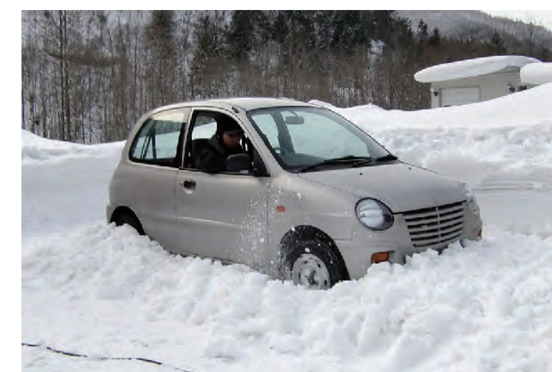
▲自動車の走行限界に関する実験(写真：吹きだまり高さ15cmの例) Experiment on the limit of a vehicle's ability to travel through snowdrifts (Photos: experiment at 15-cm-deep snowdrifts)
