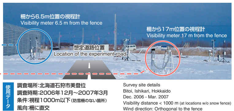
▲観測結果の一例(計測位置と視程比の関係) Example of monitoring (relationship between monitoring locations and visibility ratio)
