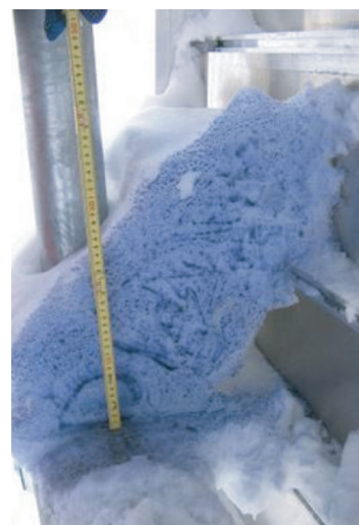
▲着雪の断面観測 Observation of accreted snow (cross section)
