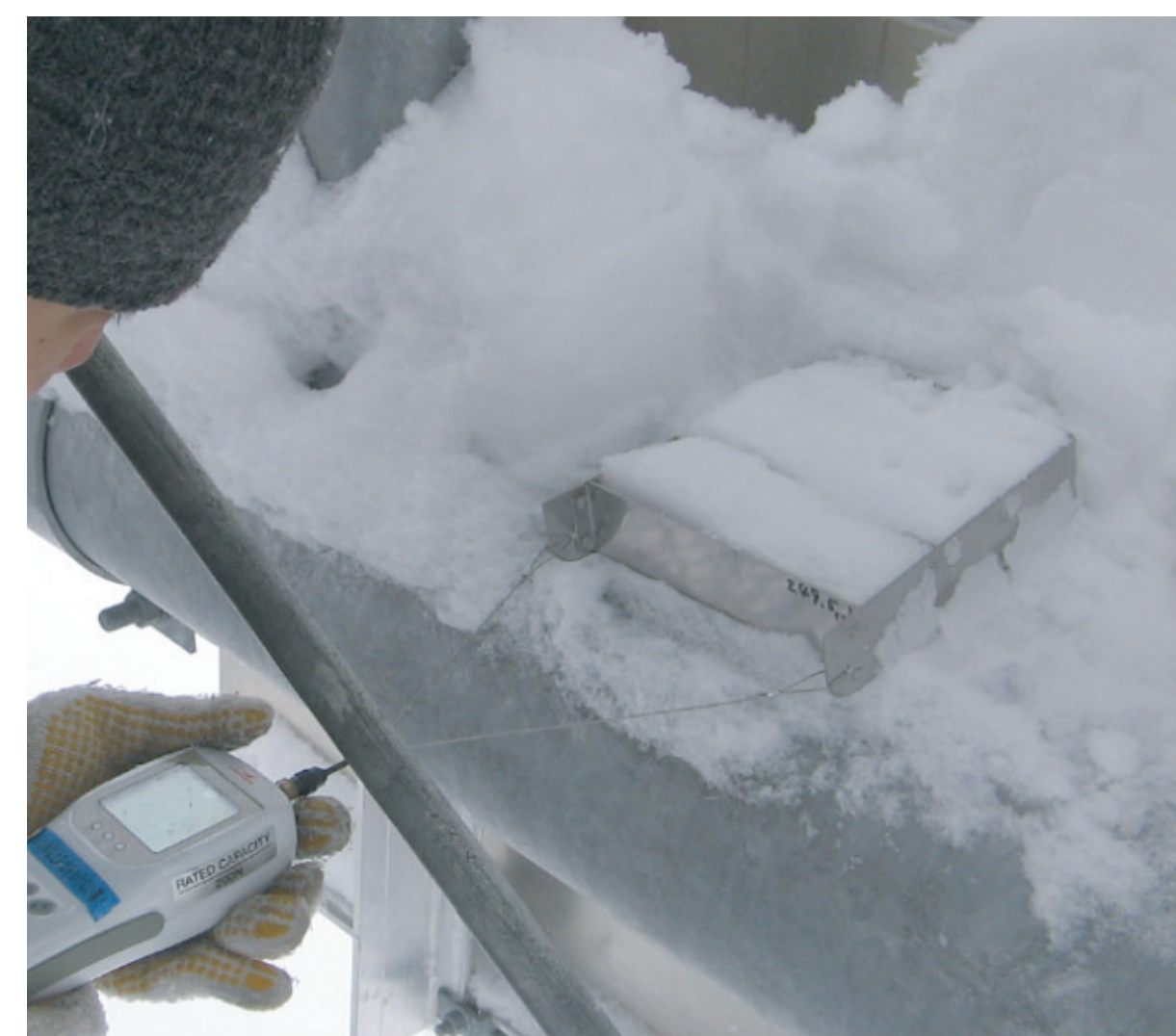
▲着雪の剪断強度測定 Shear strength measurement
