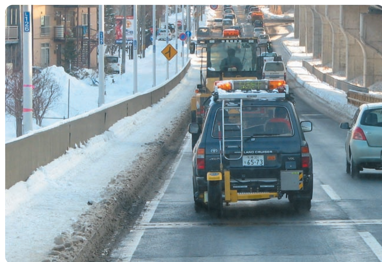
▲冬期路面のすべり摩擦の計測調査 Friction measurement on a winter road surface
