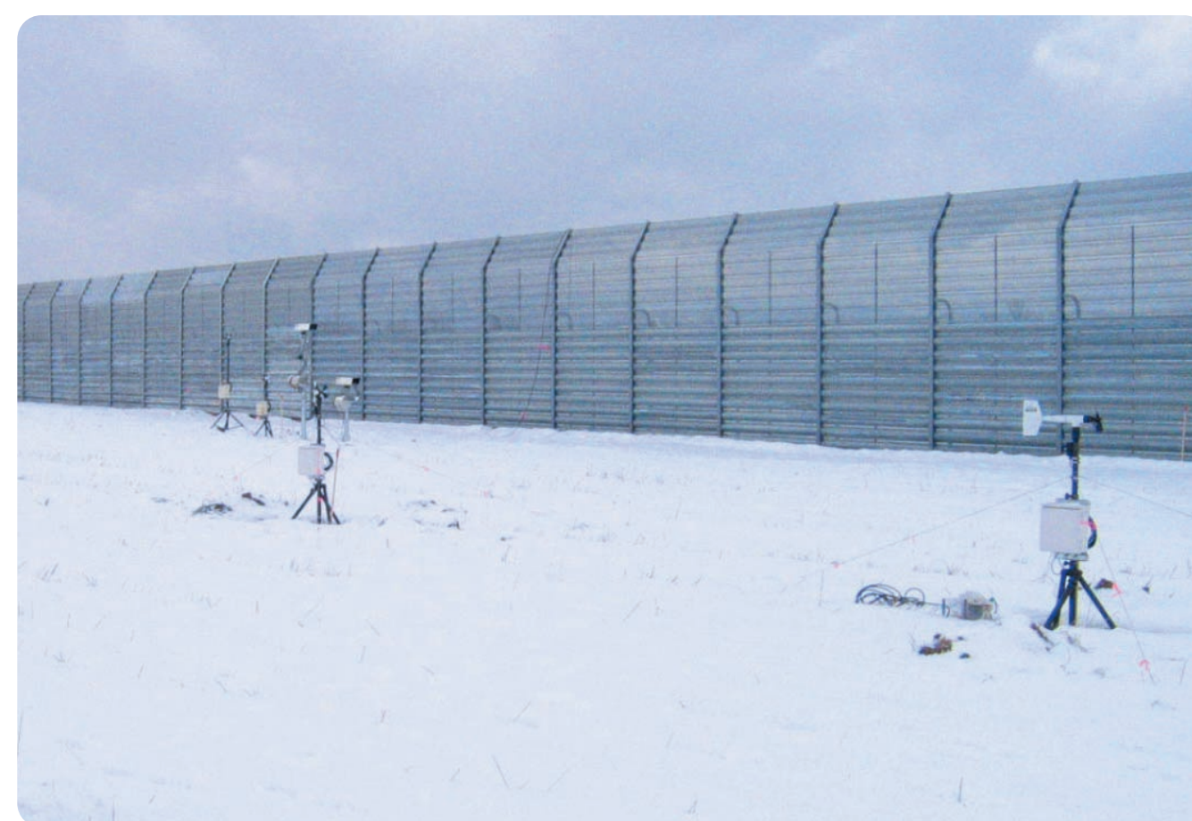
▲防雪柵の性能評価に関する観測 Observation of snow fences to evaluate their performance
