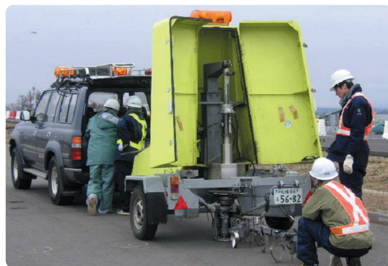
▲FWD試験による舗装体の評価 Evaluation of pavement strength by Falling Weight Deflectometer (FWD) test
