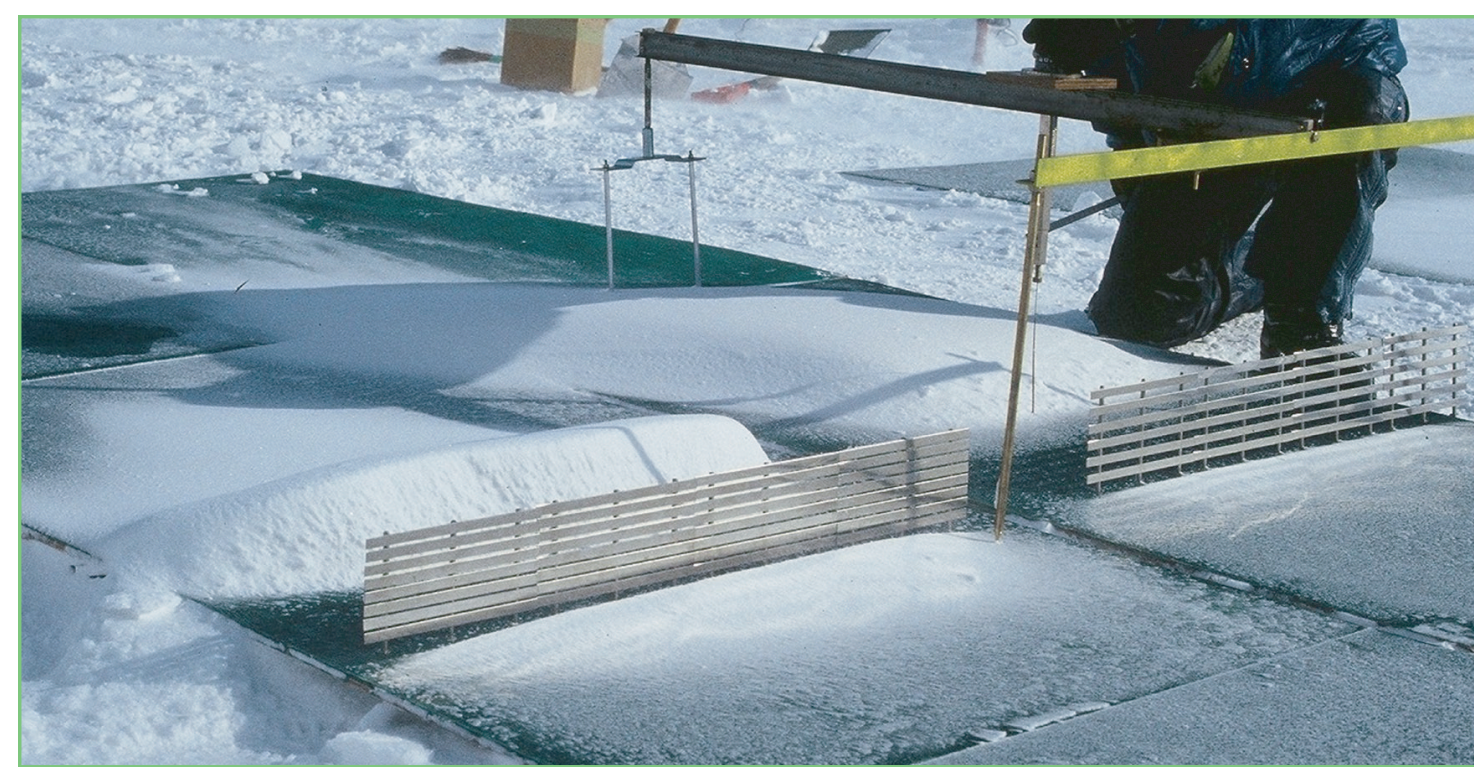
▲吹きだめ柵の野外実験 Outdoor model experiments (Collector snow fence)
