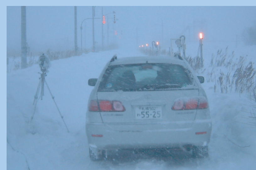
▲固定式視線誘導柱の視認性調査 Visibility test of fixed-post delineators
