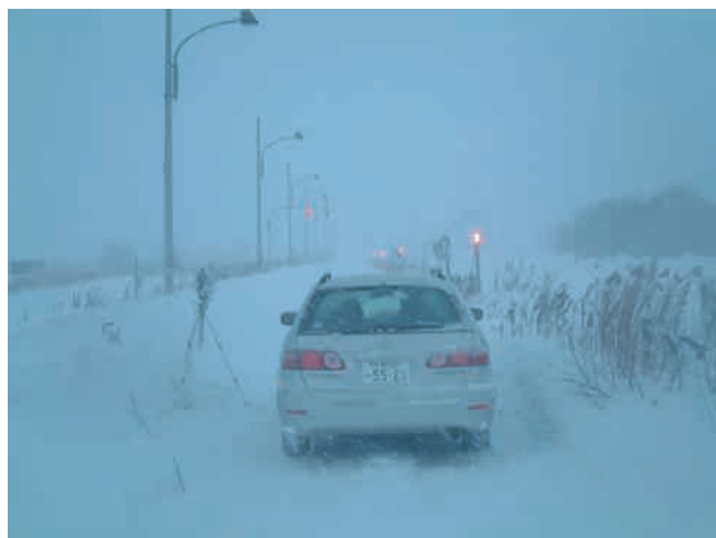
Delineator visibility test (Ishikari Blowing-Snow Test Field)
